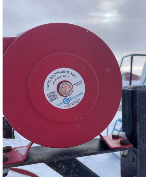
Image 2: View of Static Grounding Reel
